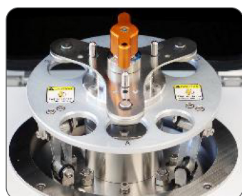
Sample grinding section Snap-lock mounting and removal of sample containers
