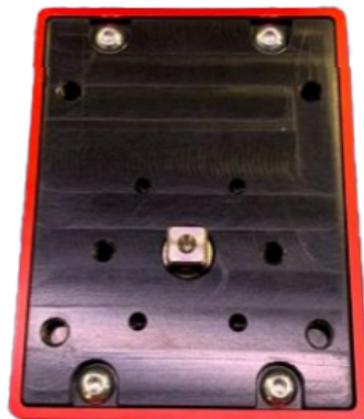
Figure 1: Retrieve the 4 screws. Tool: 2 mm. Allen Key
